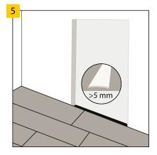
The application of the 5 mm expansion joint in the door opening between the rooms, which allows for the elimination of stresses, is recommended in the following cases: the irregular shape of the floor surface in the neighbouring rooms, the placement of heavy furniture in one of the rooms or the application of the underfloor heating only in one of the joined rooms. In the case of an area bigger than 200 m² or longer than 20 m, the expansion joint must be enlarged to 10 mm.
