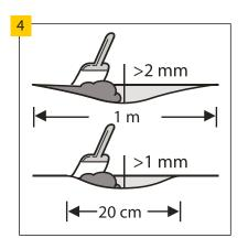
Make sure that the substrate is completely flat. All substrate irregularities exceeding 1 mm, with a length greater than 20 cm, or exceeding 2 mm with a length greater than 1 m must be levelled. Check if the use of the priming or sealing material is necessary. In order to prepare the substrate perfectly, spread the grout or the self-levelling compound on the entire surface.
