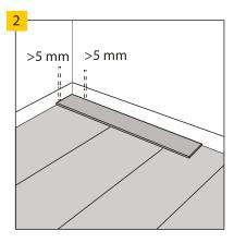
Leave 5 mm of perimeter space at the walls to allow the floor expansion. The maximum surface which can be laid without additional expansion joints is 200 m<sup>2</sup>. Above this surface, apply an additional expansion joint and enlarge all the expansion joints up to 10 mm. The maximum length of the floor surface in one direction, which can be laid without additional expansion joints is 20 m. Above this length, apply an additional expansion joint and enlarge all the expansion joints up to 10 mm.
