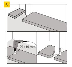
In the case of vertical pipes embedded in the substrate, leave free space around the pipes. Holes for the pipes must be drilled with a drill bit with a diameter that is bigger than the pipe diameter by 15 mm.
